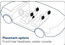
Attach the unit behind a headrest or on top of the center console.
